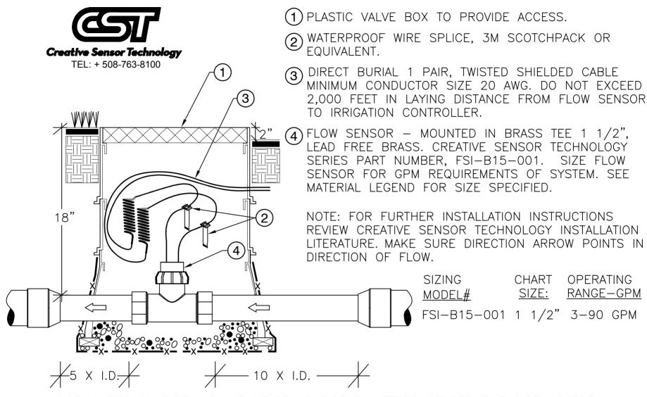
INSTALL TEE ON PIPE WITH AT LEAST 10 PIPE DIAMETERS OF STRAIGHT PIPE UPSTREAM AND 5 PIPE DIAMETERS OF STRAIGHT PIPE DOWNSTREAM OF THE SENSOR.
