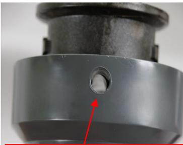
Pin goes through the sealing epoxy in the insert and is too close to the top of the tee
