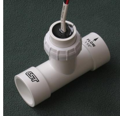
The flow sensor housing, held in place with a retaining nut, contains the detection circuitry and carries the unique four-bladed impeller on a transverse axle. The housing and mounting tee are custom molded to form an integrated measurement chamber resulting in highly accurate, repeatable flow measurements through a wide range of velocities. The axle and impeller along with the sealing o-ring are replaceable in the field.
