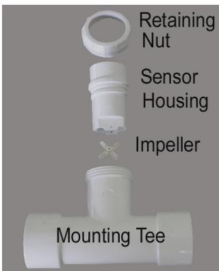
1. Always install flow arrow on the mounting tee pointed downstream. Allow 3 3/4" clearance to remove flow sensor housing from tee for service. The tee is usually installed with the housing up in the vertical or 12:00 O clock position. However, if necessary, it may be installed with sensor housing at an angle from vertical to provide clearance.
