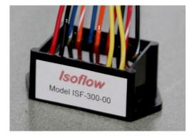
Yes, if you electrically isolate the output to each controller using an Isoflow manufactured by CST or a similar device. Every two wire flow sensor draws its power and sends its signal along the same wires. Connecting any device to two different power supplies may cause problems because of differences in the voltage levels or current cycles. The cross connection of two flow sensor inputs can cause erroneous readings and may cause permanent damage to the controller circuitry.
