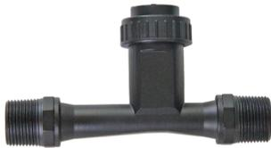
1. The unique design of the flow sensor mounting tee, serves as a flow conditioner, measuring chamber and mount for the flow sensor housing. This sensor design does not require straight lengths of pipe upstream and downstream of the sensor. Therefore, changes in pipe size or direction may be immediately before or after the sensor. In fact, solenoid valves, used as master valves may be threaded onto the downstream side of the mounting tee.
